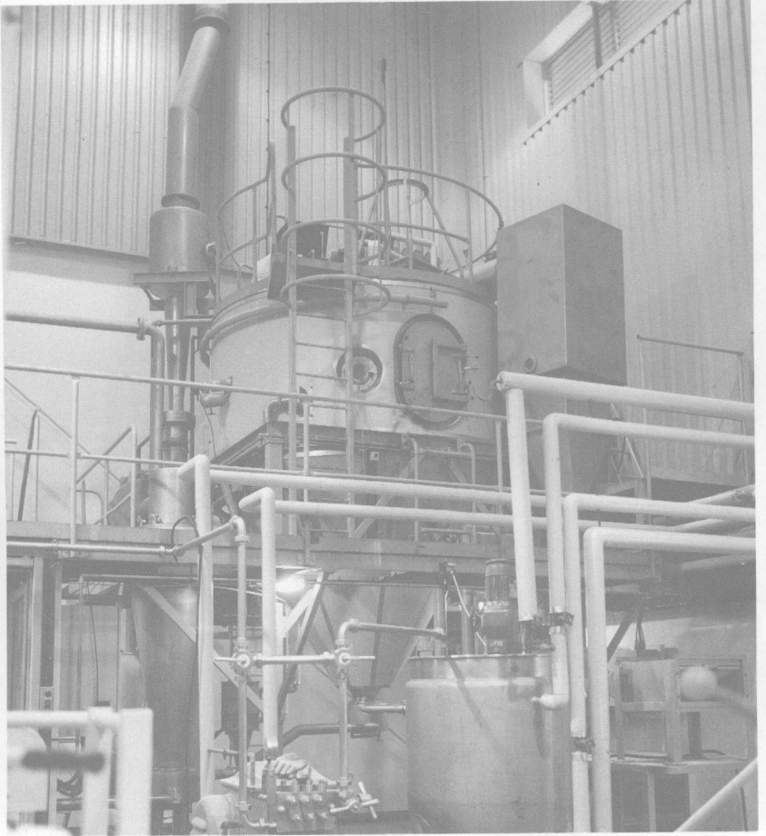
Many of the estimated 15 000 spray dryers in the world today are small units producing speciality powders (photograph by courtesy of Niro)
