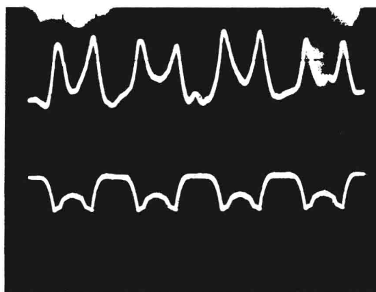
Fig. 5. Opto-Hertzian effect for nonsinusoidal laser power periodicity. Top trace is the reflected RF power, bottom trace is the laser power.
