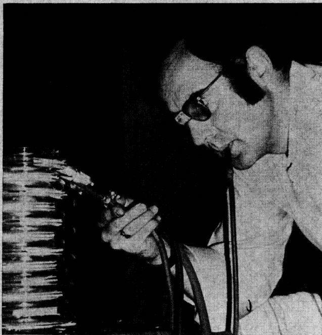
A skilled glassworker fabricating the coils of a heat exchanger made in borosilicate glass. This particular item forms part of a consignment of glass plant, made by the Process Plant Division of James A. Jobling & Co. Ltd. of the UK, for use in precious metal refining. In addition to its heat-resisting properties, the borosilicate glass must stand up to a corrosive environment involving the use of caustic soda and strong hydrochloric acid
