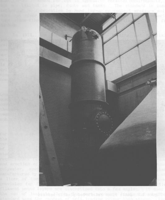
Figure 1.2: A fiber reinforced plastic vessel under hydrostatic test
