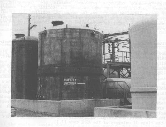
Figure 1.1: Fiber reinforced plastic acid storage tanks
