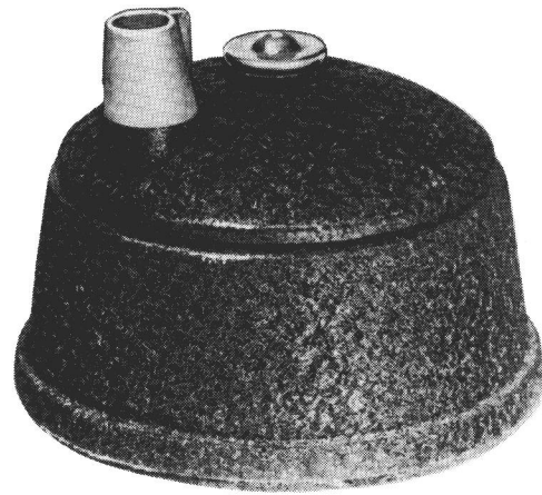
Figure 2-7. Lead pointer. Courtesy of Bruning Division, AM Corp.
