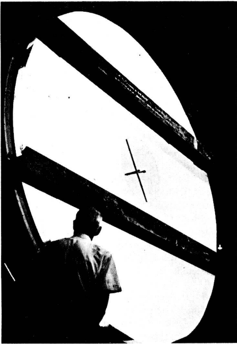
Fig. 1-1. Engineers watch the final turning of a fused silica mirror blank made for Canada's Mount Kobau National Observatory. The mirror is 157 inches in diameter and 25 inches thick. (Photograph courtesy of the Corning Glass Works.)
