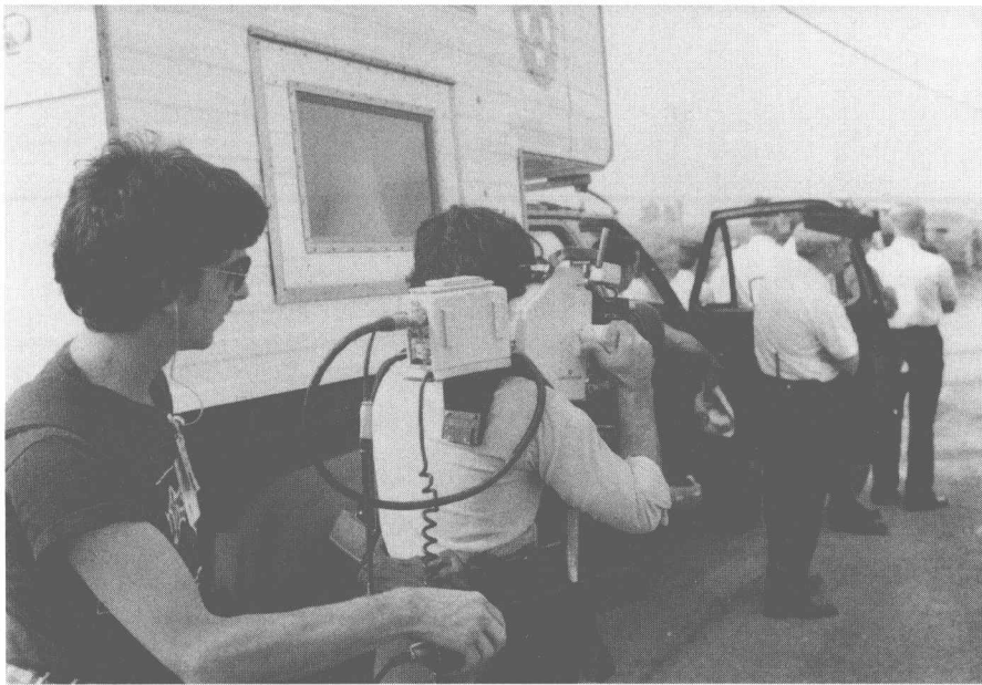
Figure 1.1 This early ENG camera, the Thompson MK-II MicroCAM, required two persons to operate it in the field. Courtesy of Larry Greene, KCBS-TV.
