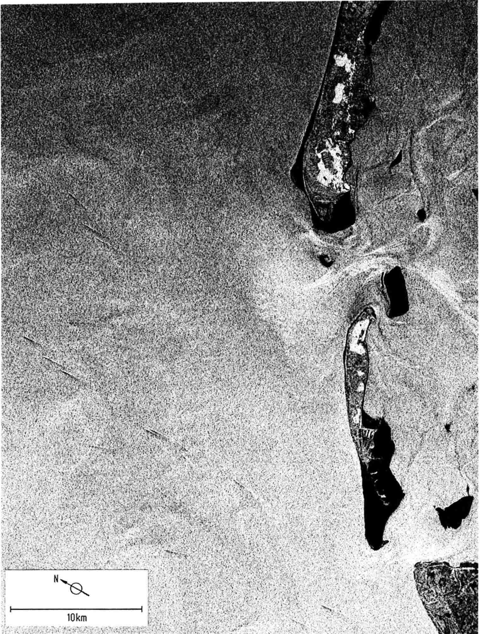
Figure 1.1: Radar image of the Dutch coast including the islands of Vlieland and Terschelling taken with the synthetic aperture radar of the SEASAT satellite on October 9, 1978 and evaluated by FVLR/GSOC. The resolution of the image is about 25 m. Image kindly provided by D. van Halsema, TNO, the Netherlands.
