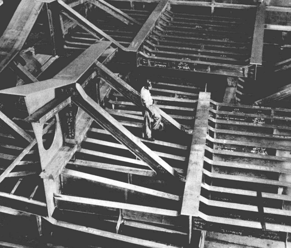
This huge welded aluminum structure, for a flight deck elevator aboard a modern aircraft carrier, measures 52 by 62 feet. By employing welded aluminum construction, 114 tons of weight were eliminated in comparison to sister ships of the same class.
