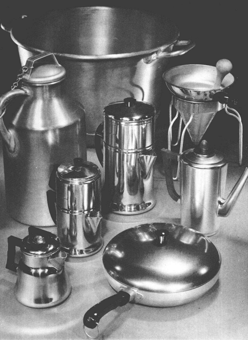
These aluminum utensils all have welded joints. Handles and bottom are welded on the tub, the handle on the milk can, leg brackets and handle sockets to the vegetable press, spouts on the coffee makers and coffee server, and the handle socket is welded to the frying pan.
