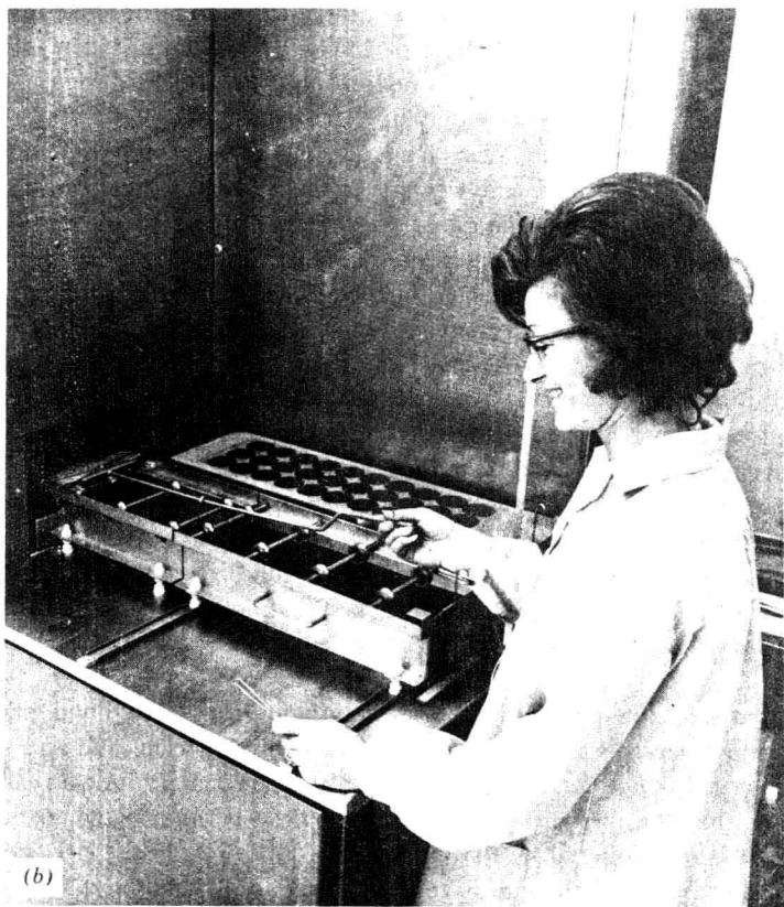
Fig. 1-1. The key to IC economy: 30 wafers, each capable of producing hundreds of ICs, can be processed simultaneously (Applied Materials AMG-500 Reactor System).
