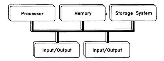
The *Processor* or *CPU* is the brain of the computer and is located within the box. The CPU receives and executes instructions from the software program loaded in the computer's memory.
