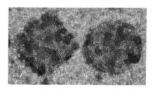
The same noninked halftone dots on the plate (plate has been washed; traces of magenta coating still visible)
