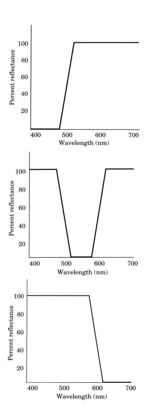
Spectrophotometric curves of a typical set of process inks: yellow (top), magenta (middle), and cyan (bottom)
