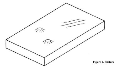
DEFINITION: a raised defect on the surface of a molded part caused by trapped gases in the part that could not escape before the surface began to "skin" during the molding process.
