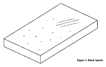
DEFINITION: small dark particles or short dark streaks on the surface of an opaque part and throughout a transparent part.
