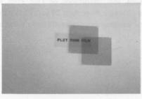
(b) Electro-optic thin films of compound (Pb,La)(Zr,Ti)O<sub>3</sub>.
