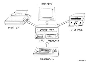
include other components too, of course). When you type a character (any letter, number or symbol) on the keyboard, a coded electronic impulse travels over a cable to the computer, where it's stored in **memory** (this kind of memory is called **RAM**).
