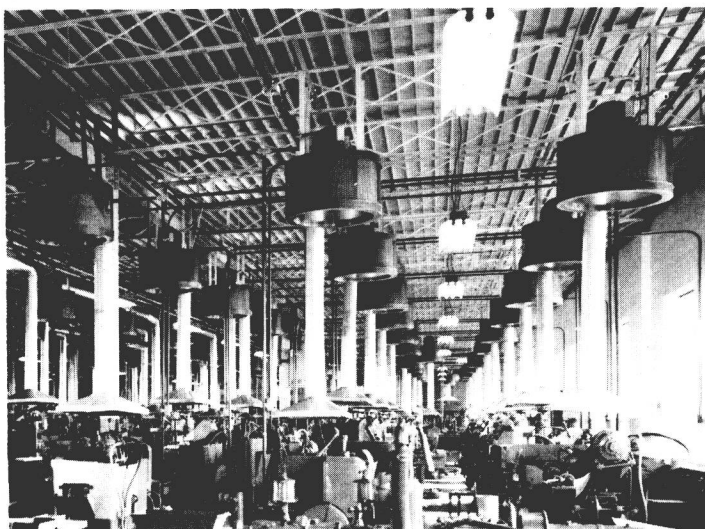
'Mistkop' filter drum as used for dust extraction from precision tap girders (right). (Belisle Filtration Ltd).
