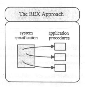
This approach forces the designer to break the application into manageable sized procedure modules whose execution and communication with other procedures is then synchronized and controlled across multiprocessor hardware by the executive.
