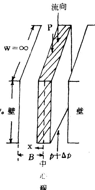
$$\therefore u = u_{\max} - \frac{g_c}{2\mu} \left[ \frac{(-\Delta p)}{y_0} + \frac{\rho g}{g_c} \right] x^2 \quad \dots \dots \dots (2)$$
