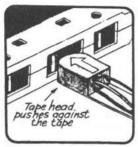
When you play the tape, the magnets make electric signals in the tape head as they move past.
