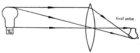
HOW THE OBJECT LENS FORMS AN INVERTED IMAGE
