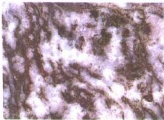
名称: 将军红 A (name): (MARSHAL RED) A 产地: 山东 (Shandong) 抗压强度: 191.70MPa 抗弯强度: 16.72MPa 编号: JGHS 115
