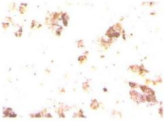
名称: 雪花红 (name): (SNOW-FLOWER RED) 产地: 山东 (shandong) 抗压强度: 106.00MPa 抗弯强度: 7.86MPa 编号: JGHS 109
