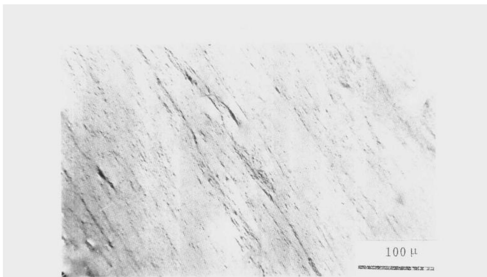
圖 1 - 3 無煙煤 有結構鏡質體（有綫狀殘痕）交叉偏光 95^{\circ} Fig. 1 - 3 . Anthracite Tellinite with filamentous relics Nicols crossed at 95^{\circ}
