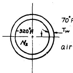
$$q = hA(70 - T_w), \text{ 或 } 70 - T_w = \frac{q}{hA} \quad \dots \dots \dots (1)$$
