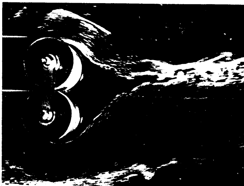
FIG. 2. Flow around two counter-rotating cylinders. "Ship of zero resistance" (PRANDTL, 1910).
