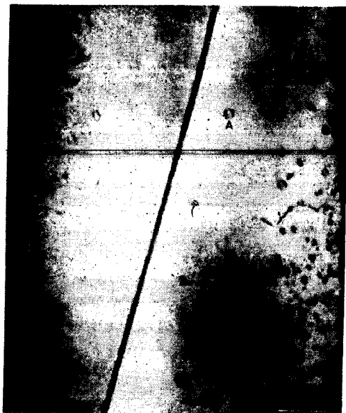
Fig. 5. Aluminum quenched from \sim 600^{\circ}\text{C} into iced brine. Note the denuded zone near the grain boundary. (After Hirsch et al. (35), courtesy Philosophical Magazine )
