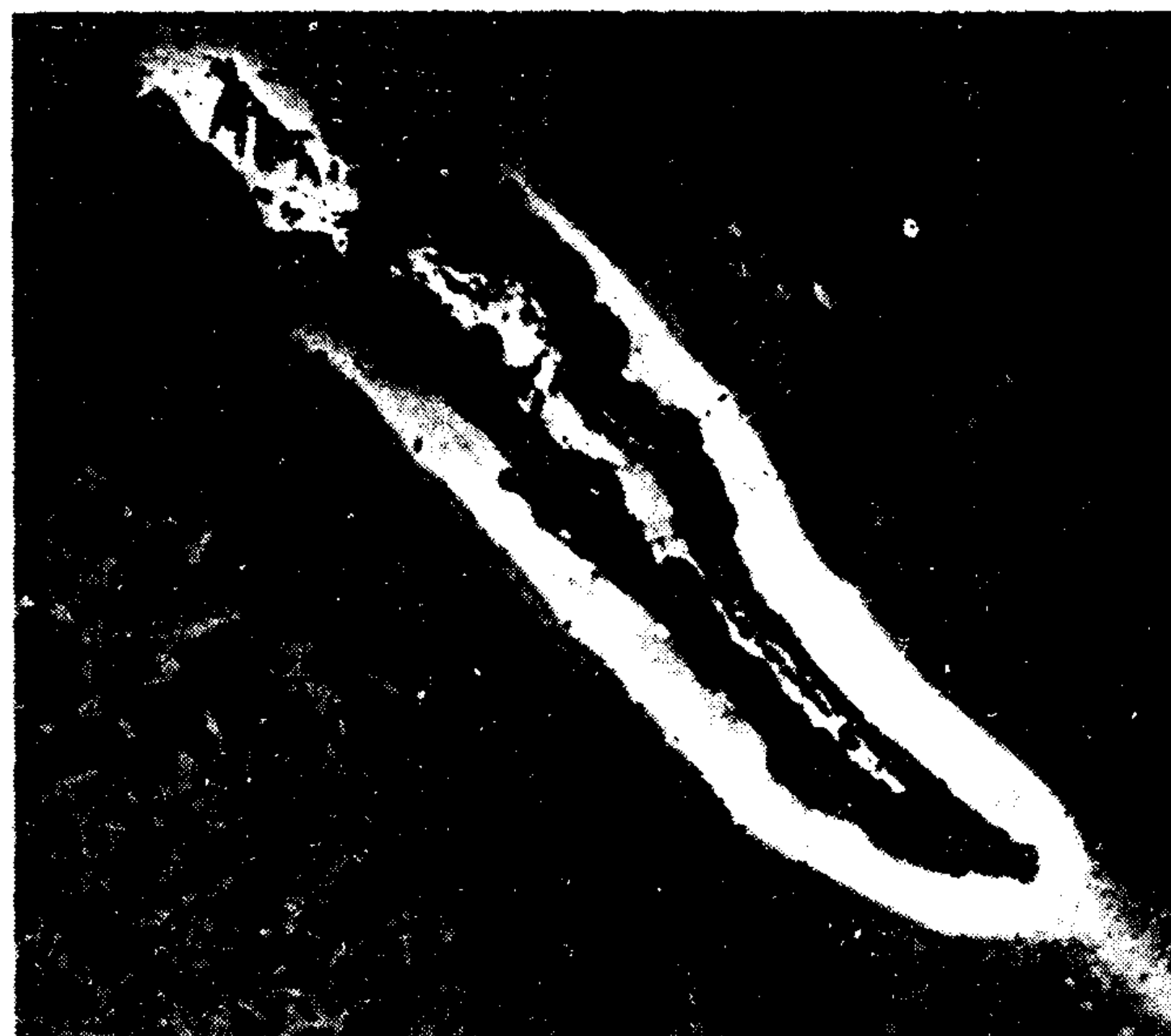
Fig. 1-13. Oxygen enrichment at a forging lap in an alloy steel revealed by Fine's alkaline chromate etch (etch No. 3i). (At 100 \times .)
