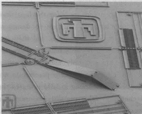
Figure 1.7 The scanning electron microscopy image of the micromirror of MEMS
