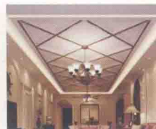
• 龙骨+长方形错层石膏板+实木菱形格栅+石膏菱形格栅
