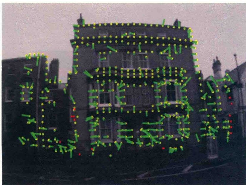
Figure 3.23 The Going Out system from Cambridge University tracks samples along strong edges in the image and compares them to a known model of the outdoor scene. Courtesy of Gerhard Reitmayr and Tom Drummond.
