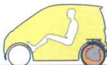
rear transverse engine and rear wheel drive 后横置后驱
