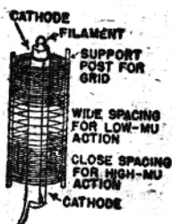
Spacing of grid wires in variable-mu tube.
