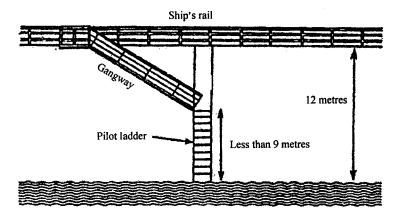
6. Gangway combined with pilot ladder. —Rules agreed between the pilots associations and the governments of most nations, stating that a pilot ladder must be between 1.5 and 9 meters in length. If the freeboard is greater than 9 meters a gangway (accommodation ladder) must be used as well as a pilot ladder.
