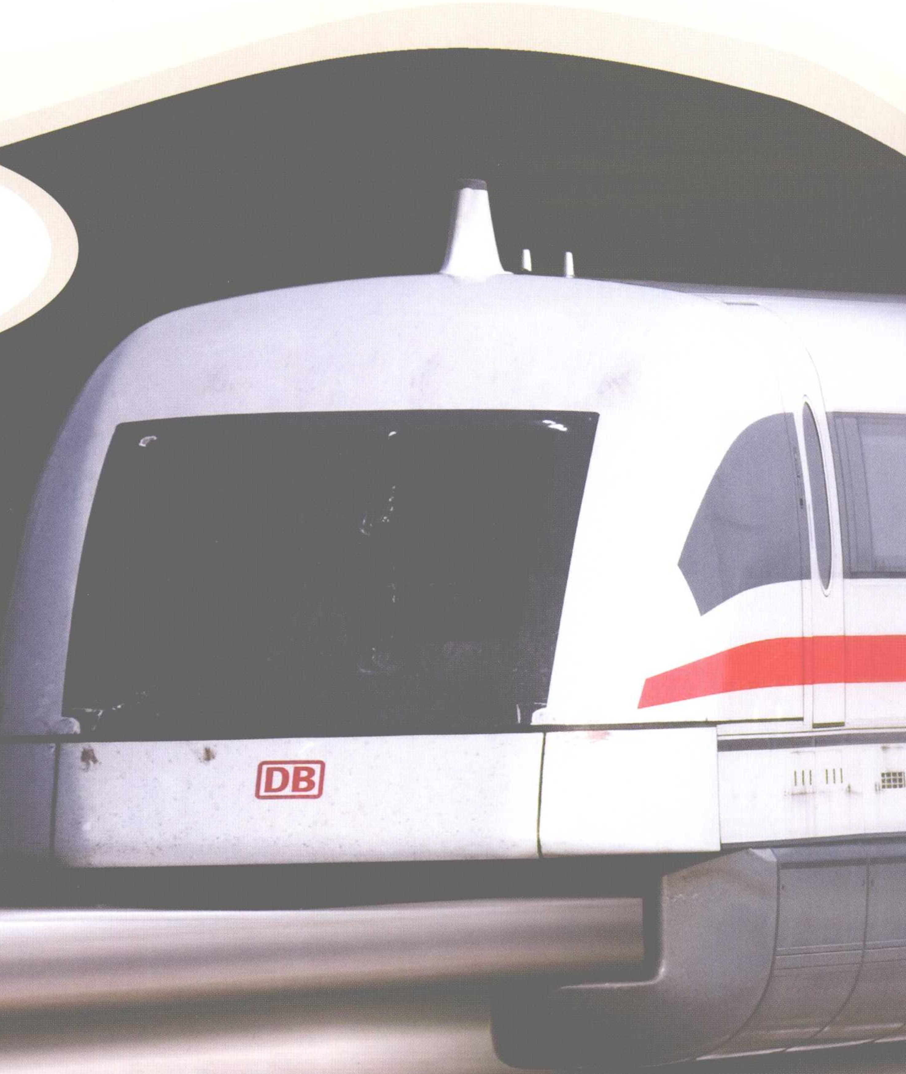
Maglev trains do not have wheels. There are powerful magnets on the track. These face magnets underneath the train. The magnets repel (push away from) each other. The magnets lift the train just above the track.
