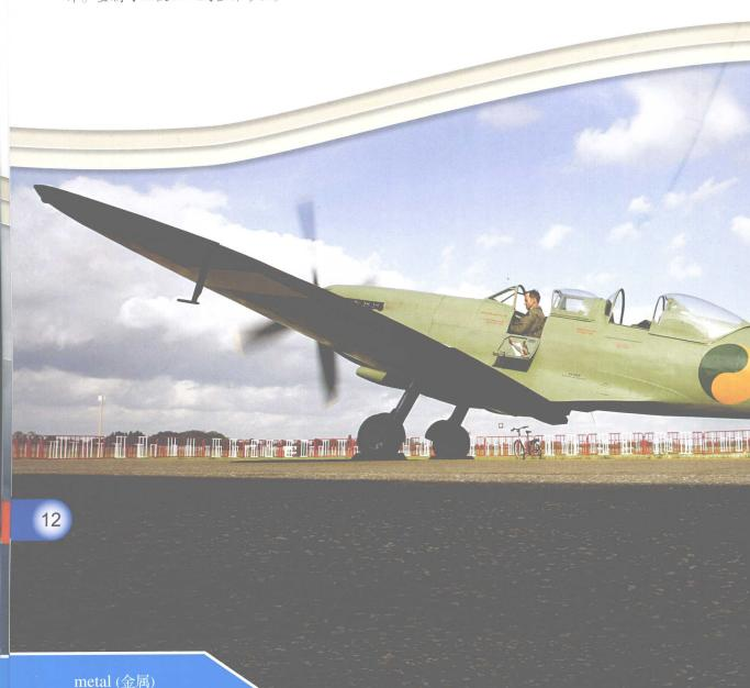
Aeroplane designers thought metal would be great for planes. They could make the metal into an aeroplane's shape. The metal would not catch fire. It would not break easily. Metal can be heavier than wood, but that was okay. Designers had built stronger engines.
