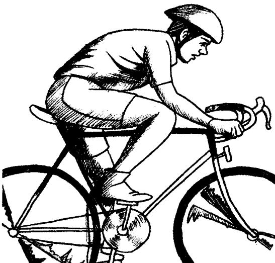
Bicycle wheels are lightweight. This is because it takes less energy to turn a light wheel than it does to turn a heavy one. Lightweight wheels still have to be strong enough to support the weight of the bicycle and the rider. This is the reason wheels have spokes—to add strength.
