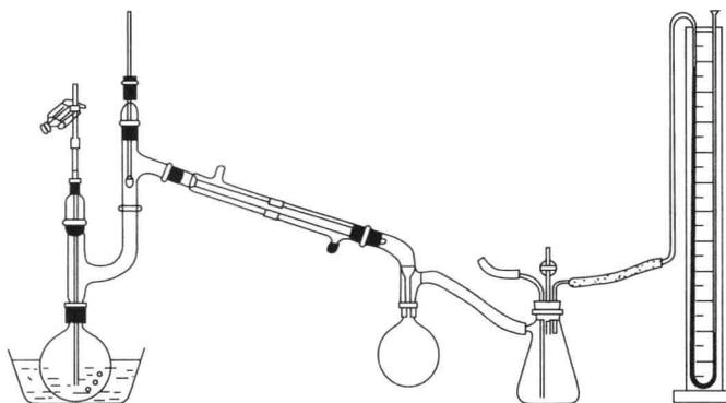
Figure 1.9 Vacuum Distillation Apparatus
