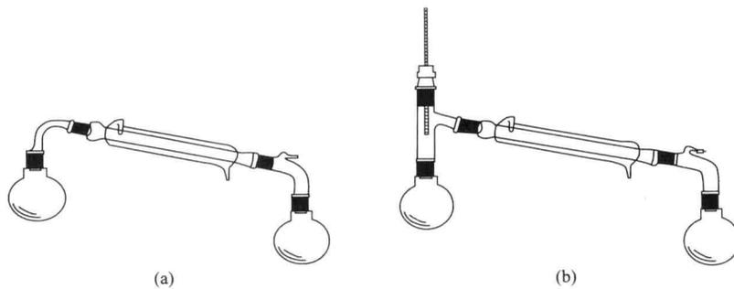
Figure 1.6 Distillation Apparatus
