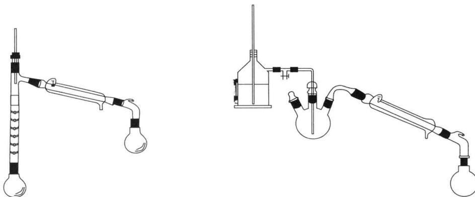
Figure 1.7 Fractional Distillation Apparatus
