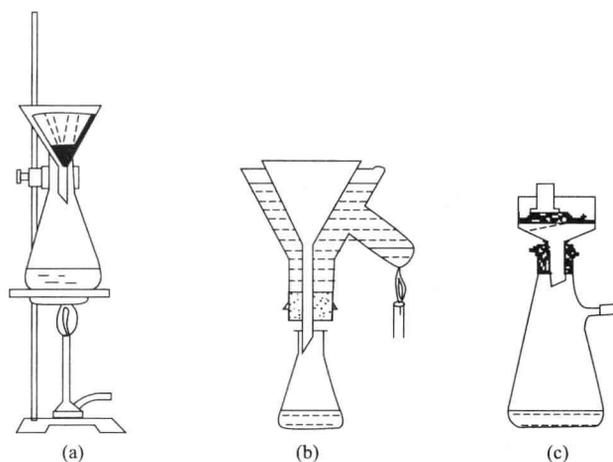
Figure 1.11 Heat Filtration and Vacuum Filtration
