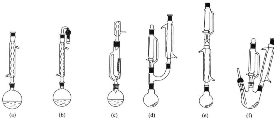
Figure 1.5 Reflux Apparatus
