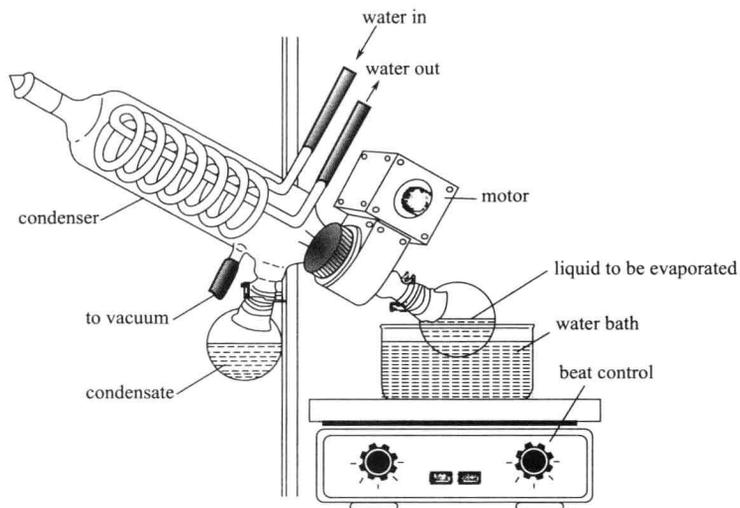
Figure 1.10 A Rotary Evaporator with Condenser and Receiving Flask
