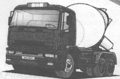
Concrete mixer 搅拌车
