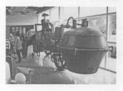
1771 in Paris, where a French engineer named Fardier De Cugnot built the first self-propelled vehicle, a heavy, three-wheeled, steam-driven carriage with a boiler that projected in front, its speed was only 2.3mph.
