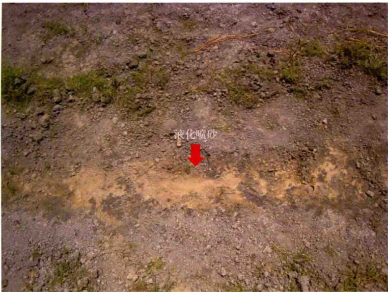
(a)液化喷沙裂隙长约 1.5m
