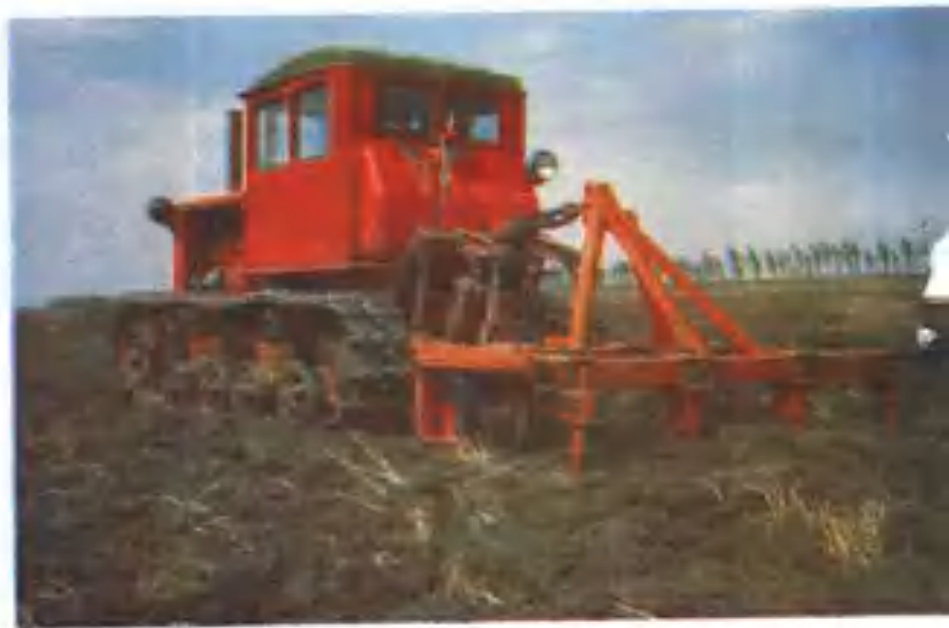
Subsoil Plough improving cold and clay meadow soil. Changan Countryside, Fujin County, Heilongjiang Pro- vince
