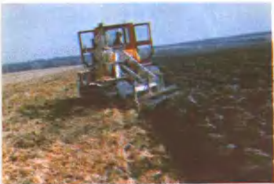
Subsoil Plough improving Planosol with poor physical chemical properties. 853 State Farm, Baoqing County, Heilongjiang Province.
