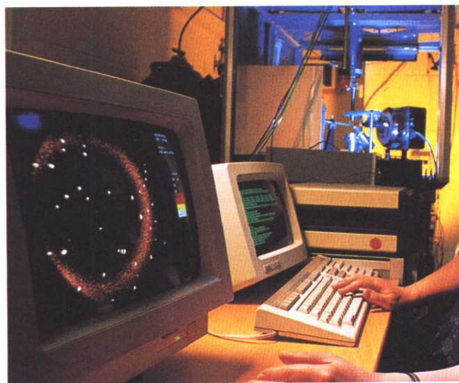
Figure 1.4 A modern X-ray crystallography instrument, used for studying crystal structure.
