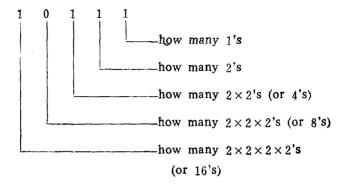
Thus, in the binary scale, 2 is expressed as 010, 3 is given as 011, 4 is represented as 100. This scale is perfectly adapted to the "off-on" pulses of electricity, so it is widely used in electronic computers.
