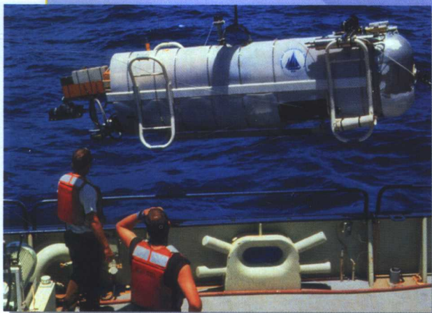
DSL-120 gets lowered over the side of the research ship.
