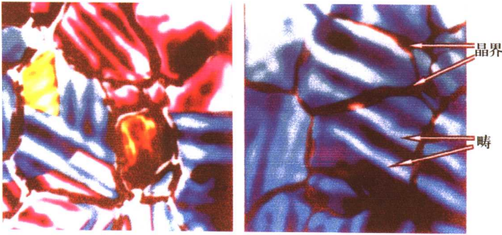
Fig.1-53 Electron acoustic image of grain, grain boundaty and donain structure in BaTiO 3 ceramics (the sample without polish and etching)
