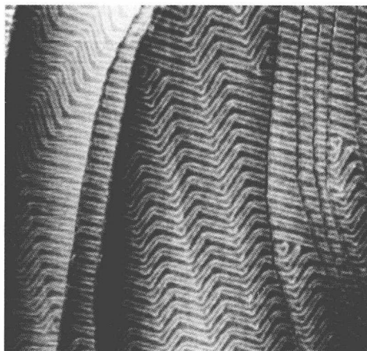
Figure 2 STM image of the Au(111)- (22 \times \sqrt{3}) herringbone reconstruction. Obtained from http://ipn2.epfl.ch/LESEN/jvb/collection/coll_au111.htm .
