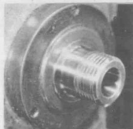
▲舊車床之螺絲式主軸端
