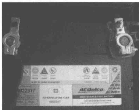
图 1-33 安装负极电缆夹
