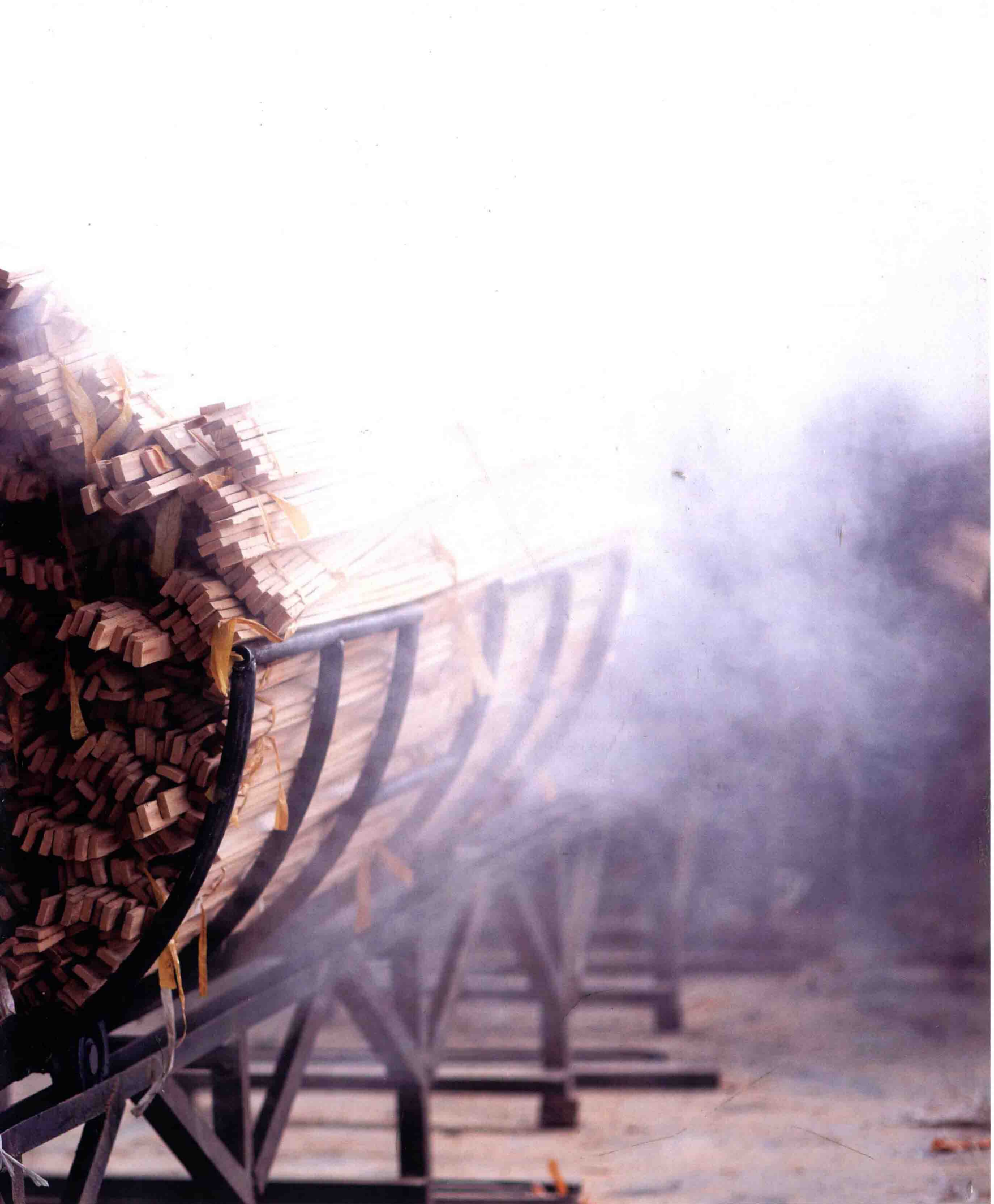
经过高压蒸汽处理的竹板条 Bamboo battens after being steam-treated in a pressure tank
