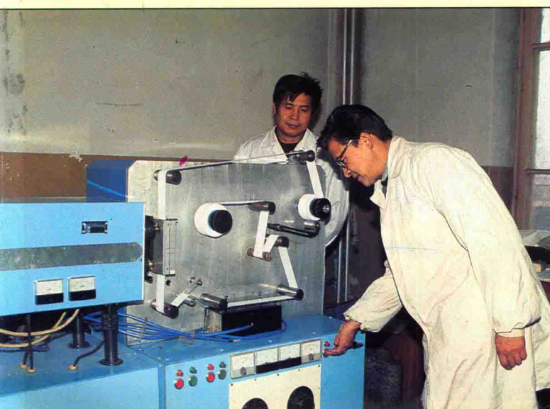
水松紙激光打孔機在試車 The laser perforator of China cypress paper in its test run
