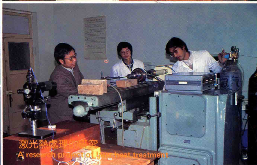
新研製的激光掃描尺寸自動檢測儀在進行測試實驗 The newly developed laser scanning automatic size tester in testing
