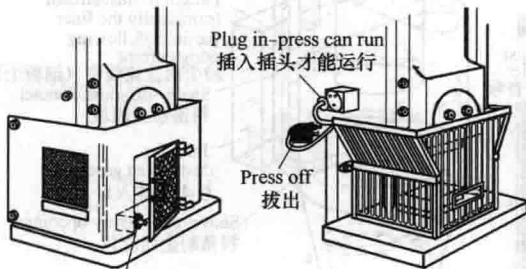
(a) Spring-type interlock shuts off power to machine when guard door is opened 防护罩门打开时，弹簧式互锁开关将切断机器电源
